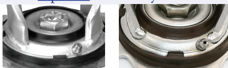
Raceway Seals (L) Thermo-plastic - up to 140° F
