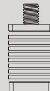
R6 (ADS7615) Fit 1-1/2 Square Tube Exp. 1.426 - 1.589 1/4 Square Metal Top Round Rubber 1/4 Square Metal Base
