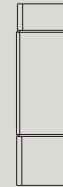
T2 (ATR7278) Fit 7/8 Square Tube Exp. 0.852 - 0.927 13/32 Square Top Square Rubber 3/4 Square Base
