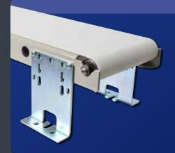
Frame Mounted version attaches directly to the frame with mounting holes every 3". T-slot mounted version attaches to 1" Side Rails, 2" Side Rails, the Single T-slot and the Multi T-slot. Brackets are universal and work on either side of conveyor. Compatible with any standard cleat height.
