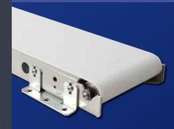
Attaches directly to the conveyor frame. The frame has mounting holes every 3". Brackets are universal and can work on either side of the conveyor. Cannot be used with cleated belts.
