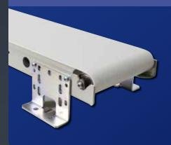
Frame Mounted version attaches directly to the frame with mounting holes every 3" (compatible with cleats 1" or lower). T-slot mounted version attaches to 1" Side Rails, 2" Side Rails, the Single T-slot and the Multi T-slot (compatible with cleats 1/2" or lower). Brackets are universal and work on either side of conveyor.
