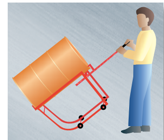
For proper use, simply: 1 ) lean cradle against drum with nose prongs astride bottom chime; 2 ) pull out handle and position hook over chime of drum; 3 ) pull back on handle and drum will seat onto prongs for tipping into horizontal position.
