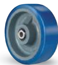
Series SP—Poly-Soft® Liquid cast 82A polyurethane tread chemically bonded to heavy duty iron center. Tread formula provides quiet operation, excellent rollability, and repels foreign objects & debris (F.O.D.). Page 77.
