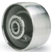
Series FS—Forged Steel Highest capacity, solid web wheels drop forged to provide tensile strength in the 75,000 psi range. Some sizes available V-Grooved (FV) or Flanged (Suffix-F). Page 72.
