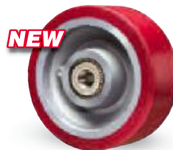
Series STR—Super Ultralast™ The new ultimate urethane with a 1" thick tread bonded to the super duty drop forged steel center. Page 76.
