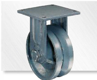
Maxi-Duty Rigid models feature reinforced 3/8" x 5" plate steel legs, continuously welded inside and outside to 1/2" thick mounting plates.
