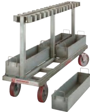
Fig. 1177 Stainless Steel Cart with brackets along top frame for holding bottle capping spindles submerged in removable oil pans.
